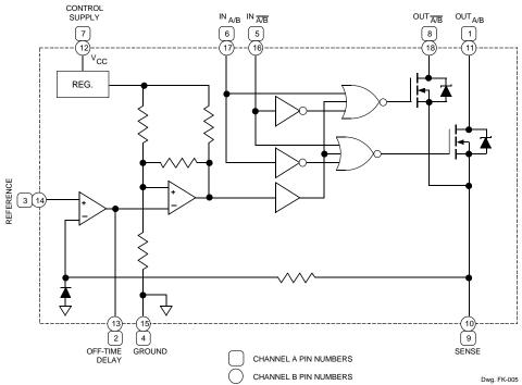
Note that channels A and B are electrically isolated.
