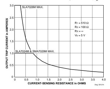
FIGURE 3. CURRENT-SENSING RESISTANCE
