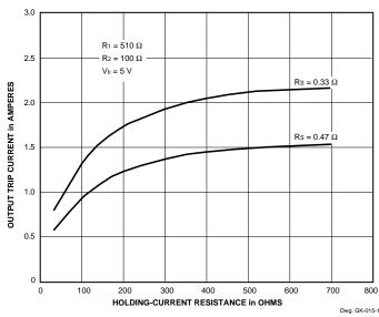
FIGURE 5B. HOLD-CURRENT RESISTANCE (SLA7026M)
