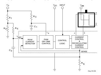
FIGURE 2. PWM CONTROL (RUN MODE)
